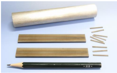
Fig. 1 Fe-Ga alloy, D22 L120 mm rod and its cut into plates.
